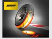
What is it? Casing construction allowing to reduce inflation pressures for track days
