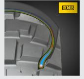
What is it? Casing reinforced with a spiral overlay of steel or aramid.
